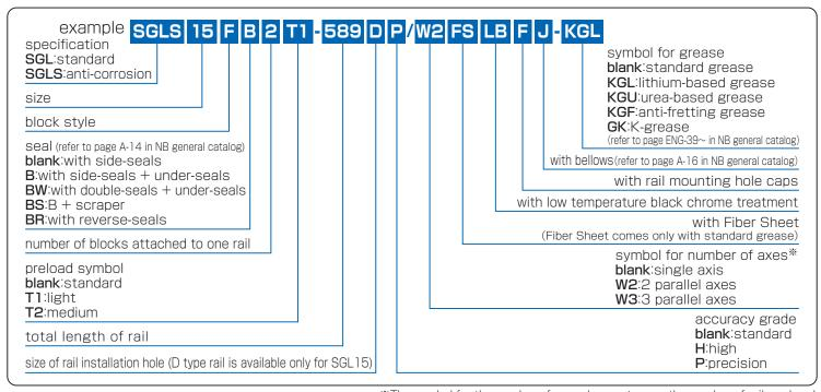
\*The symbol for the number of axes does not mean the number of rails ordered.
